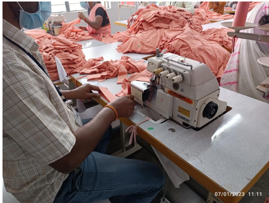
8.Sewing Machine with Eye Guard.jpg
